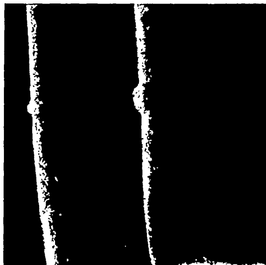
(b) After exposure of wires to exhaust-gas stream from apparatus B. Beads on wires are resistance-welded junctions.
