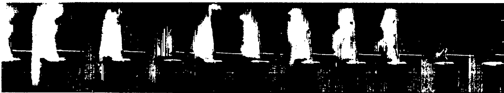
Fig.16 Fuel spray with an air jet impinging at right angles from the right. Fuel-injection pressure, 1,000 pounds per square inch. Air-jet injection pressure, 200 pounds per square inch. Chamber-air density, 0.076 pounds per cubic foot.
