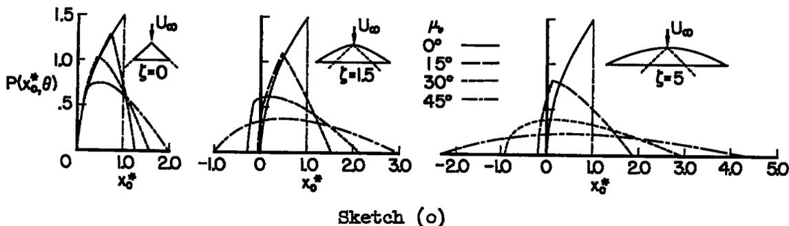
In sketch (o), these loadings are drawn for the three members of the family corresponding to  $\zeta = d/l = 0, 1.5, 5$ , with  $\beta = 1$  and  $\mu_0 = 0^\circ, 15^\circ, 30^\circ, 45^\circ$  in each case. The dimensionless quantities plotted are
