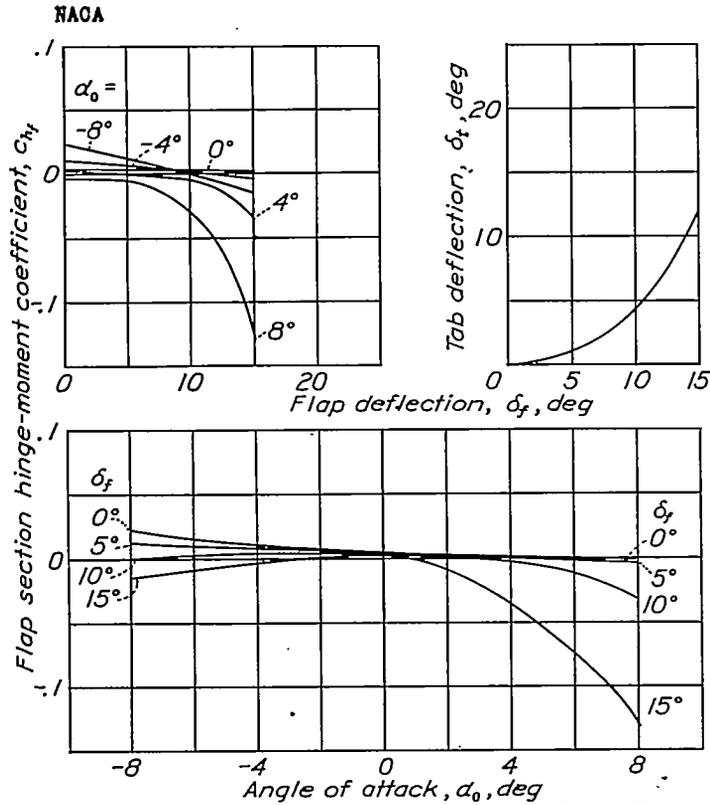
Figure 8.- Hinge-moment characteristics of a 0.30c flap having 0.495 $c_f$  overhang, blunt nose, and sealed gap and a 0.20 $c_f$  differential balancing tab. NACA 0009 airfoil.
