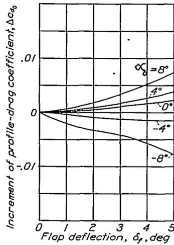
Figure 6.- Increment of profile-drag coefficient caused by flap deflection. Blunt nose, sealed gap, 0.485c of overhang.
