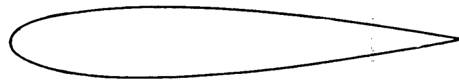
NACA 00XX series Geometric twist of 0^\circ to obtain zero aerodynamic twist at M=0.30 .
