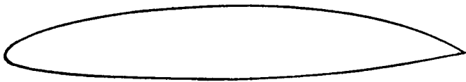
NACA 16-5XX series Geometric washout of 1^\circ to obtain zero aerodynamic twist at M=0.30
