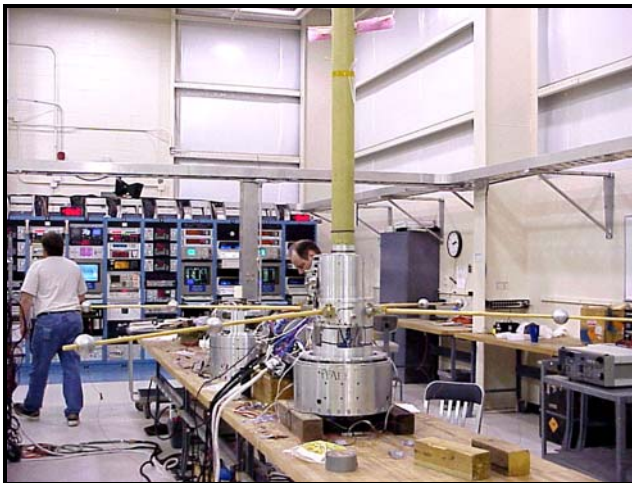
Figure 2.4.1 The Very Complex Pfaff Payload Used Extended Booms to Investigate Sporadic E Events in the Ionosphere; Pfaff 21.126 Launched on 26 June 2001.
