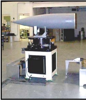
Figure 6.2.1-1 Airborne Mark 8 Mass Properties Measurement System at WFF
