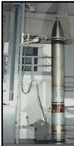
Figure 6.2.5-1 Bend Test Fixture at WFF
