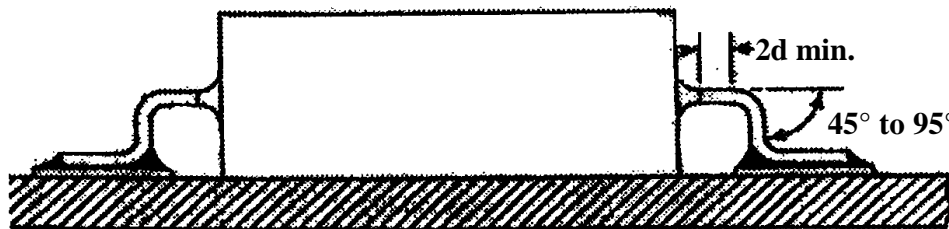
Figure 8-11. Bend Angle
