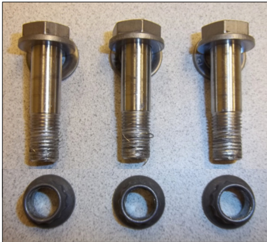
Figure 8. Tension load only bolts with thread shear failure.
