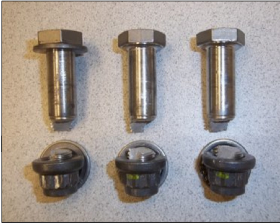
Figure 9. Tension load only bolts with bolt failure in the threads.
