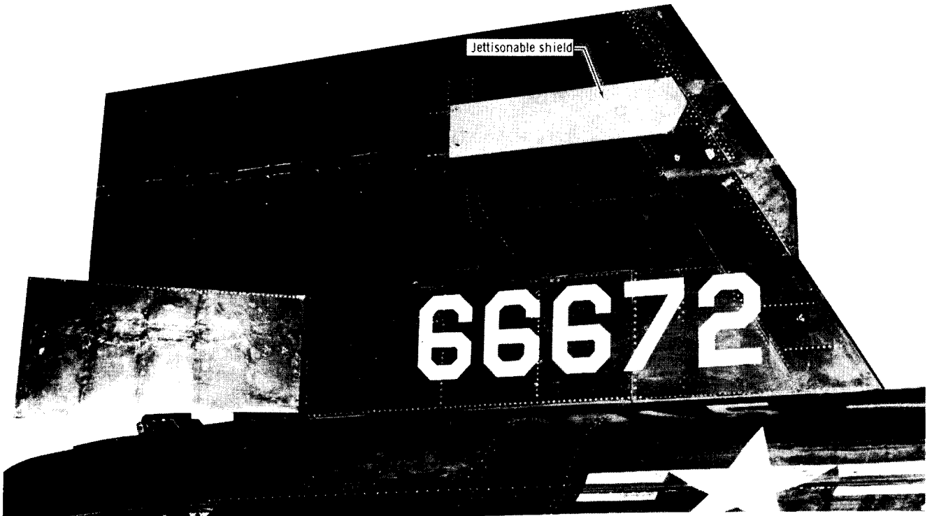
(b) Jettisonable shield installed on vertical tail.
