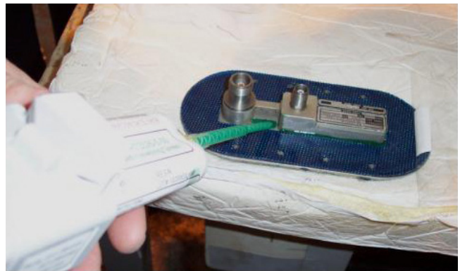
Figure 6-4. Application of Self-Leveling Green Sealant
