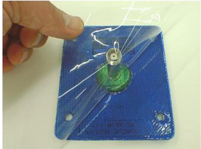
Figure 6-3. Removal of Release Film From Gasket
