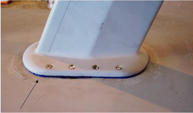
Figure 6-6. Typical Gel Squeeze-Out Around Perimeter of Antenna
