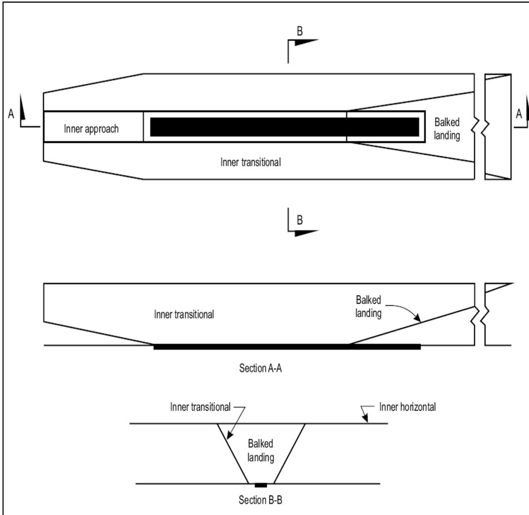
**Figure 4-4. Inner approach, inner transitional and balked landing obstacle limitation surfaces**
