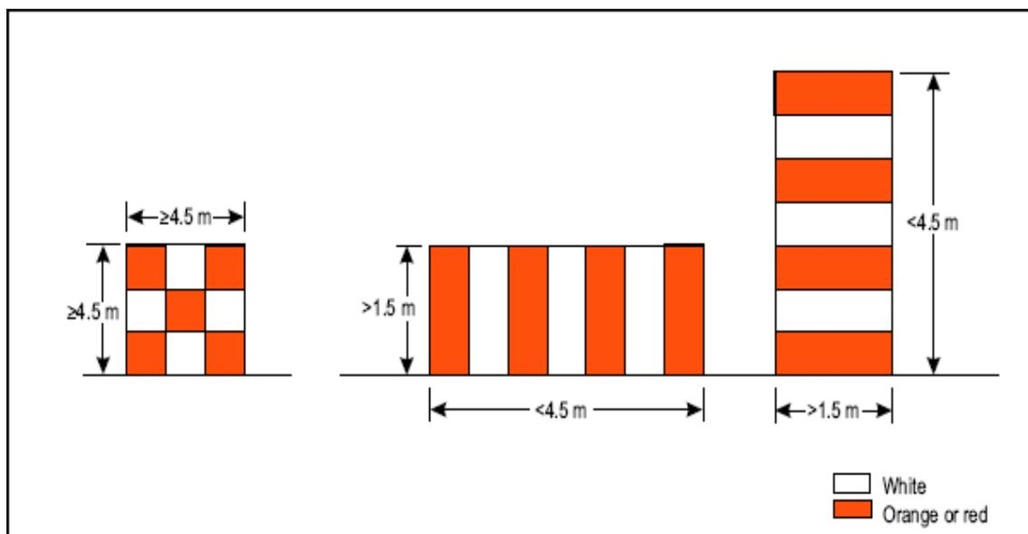
**Figure 6-1. Basic marking patterns**
