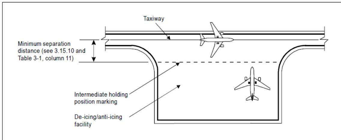
**Figure 3-4. Minimum separation distance on a de-icing/anti-icing facility**
