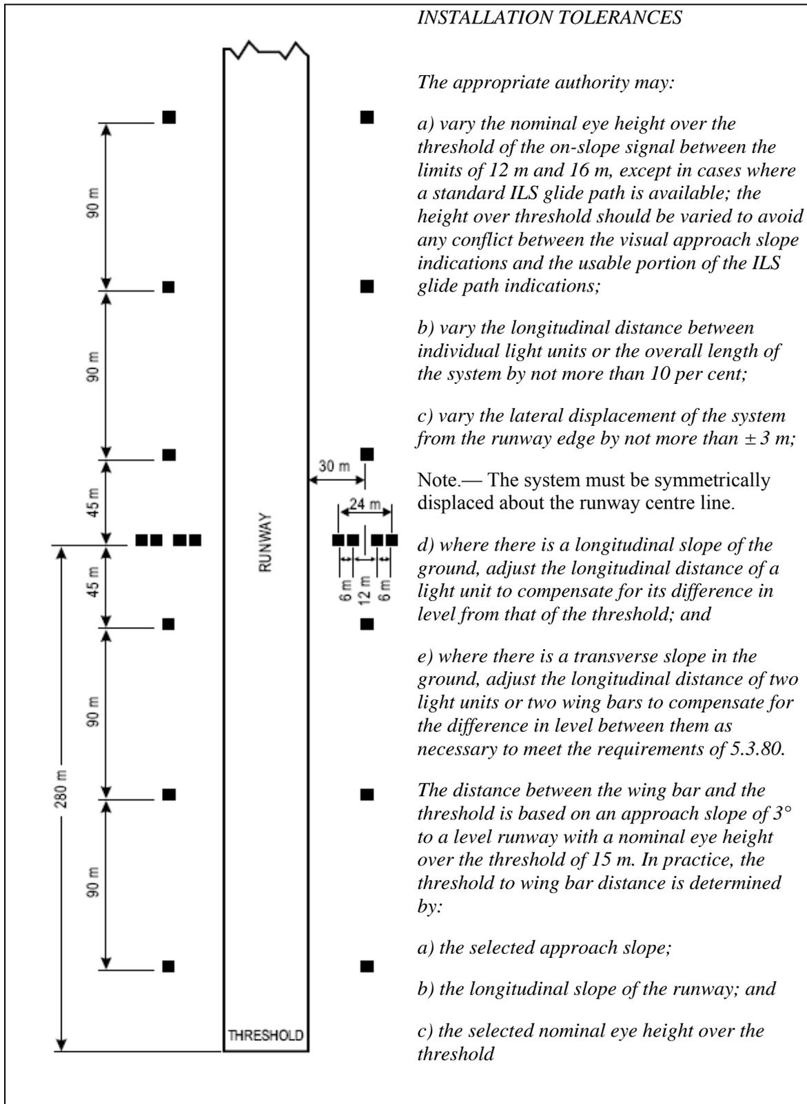
**Figure 5-19. Installation of light units for T-VASIS**
