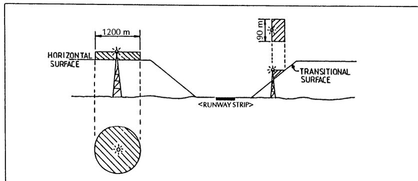
**Figure 4-8. Shielding – transitional and horizontal surface.**
