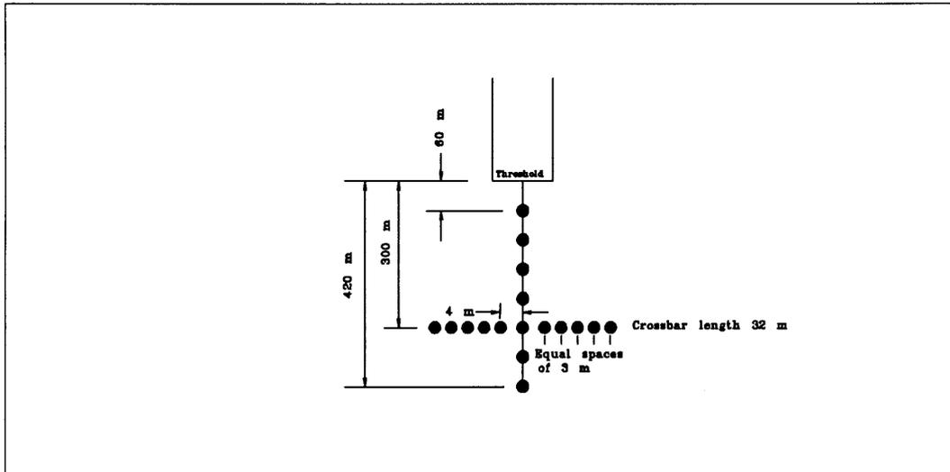
**Figure 5-12A. Low intensity approach lighting system 1 Bar**
