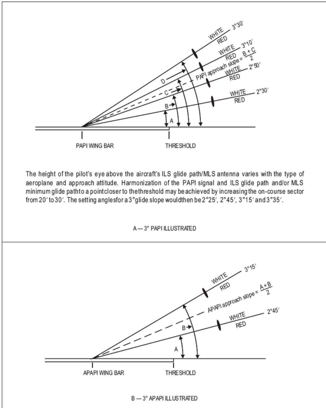
**Figure 5-23. Light beams and angle of elevation setting of PAPI and APAPI**
