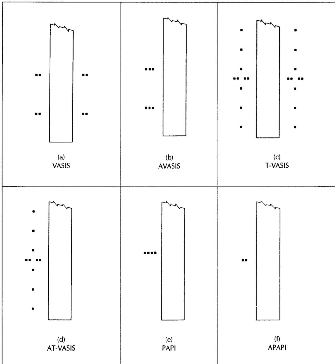
**Figure 5-16. Visual approach slope indicator systems**
