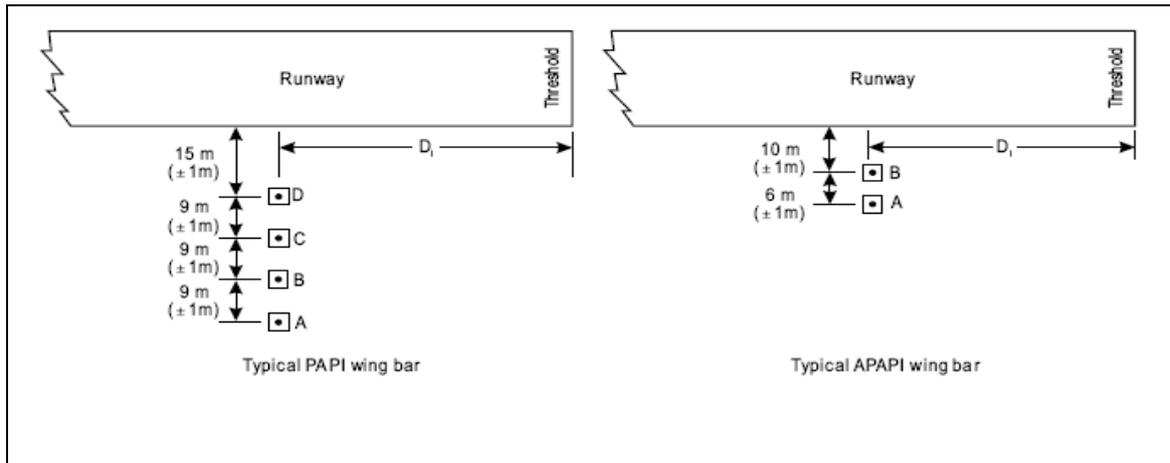
a) Where a PAPI or APAPI is installed on a runway not equipped with an ILS, the distance D1 should be calculated to ensure that the lowest height at which a pilot will see a correct approach path indication (Figure 5-23, angle B for a PAPI and angle A for an APAPI) provides the wheel clearance over the threshold specified in Table 5-2 for the most demanding amongst aeroplanes regularly using the runway.
