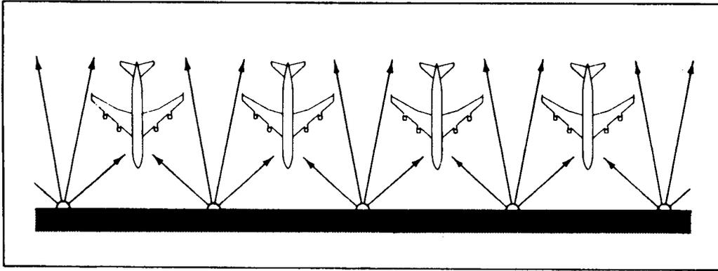
Figure 5-26b. Typical arrangement and aiming for nose-in parking
