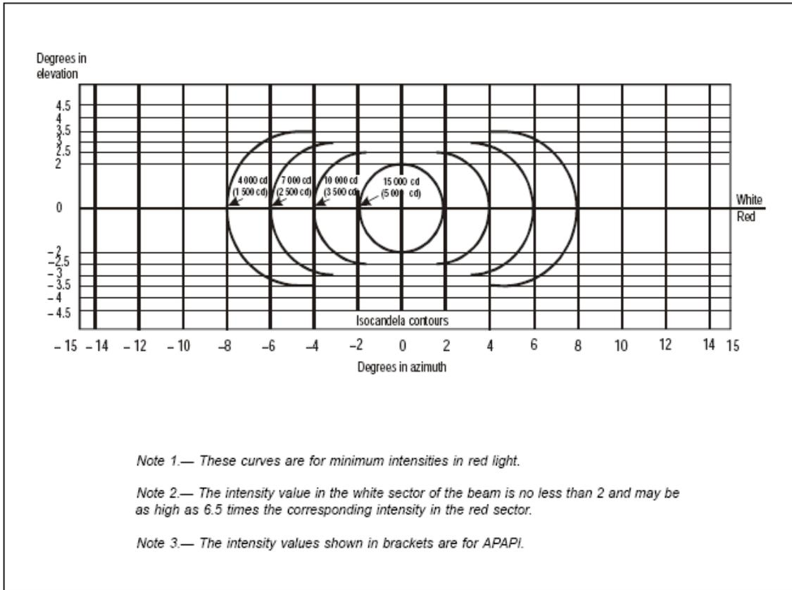
**Figure 5-22. Light intensity distribution of PAPI and APAPI**
