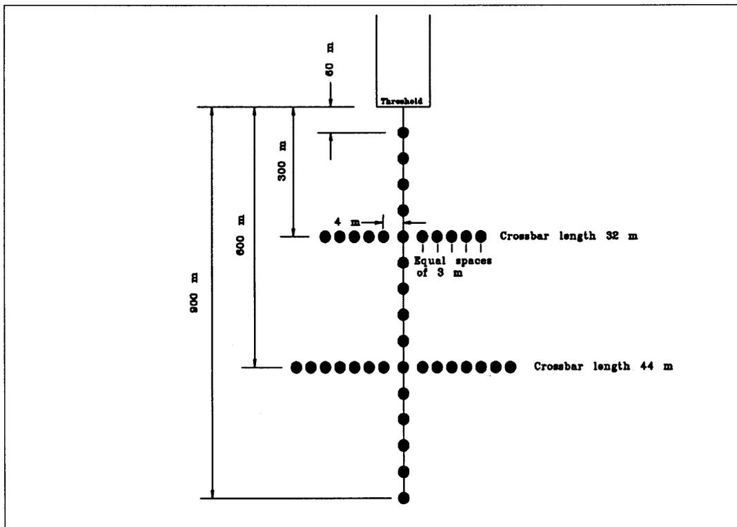
**Figure 5-12B. Low intensity approach lighting system 2 Bar**
