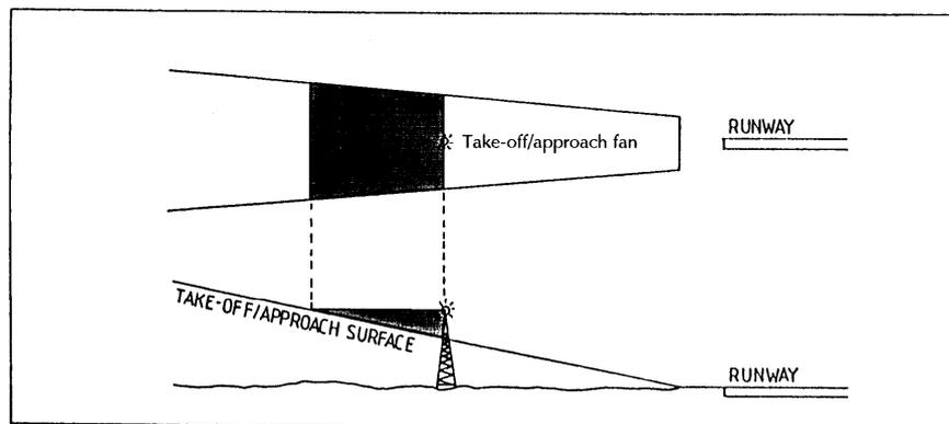
**Figure 4-7. Shielding – approach and take-off surfaces**
