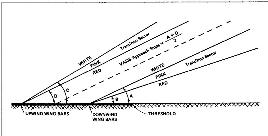
**Figure 5-17. Light beam and angle of elevation setting of VASIS and AVASIS**
