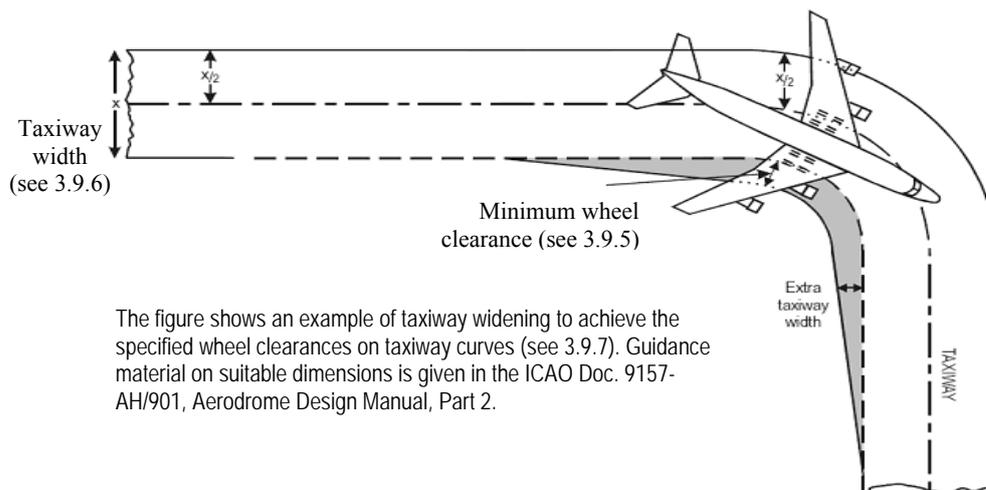
The figure shows an example of taxiway widening to achieve the specified wheel clearances on taxiway curves (see 3.9.7). Guidance material on suitable dimensions is given in the ICAO Doc. 9157-AH/901, Aerodrome Design Manual, Part 2.
