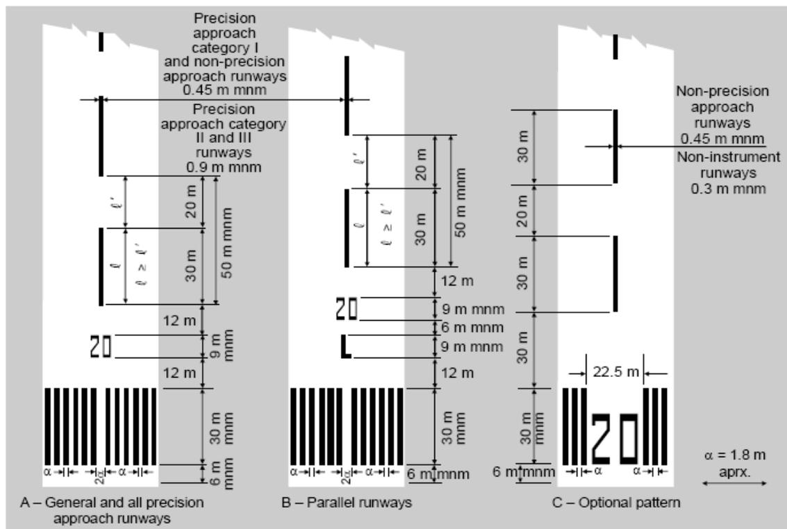
**Figure 5-1. Runway designation, centre line and threshold markings**
