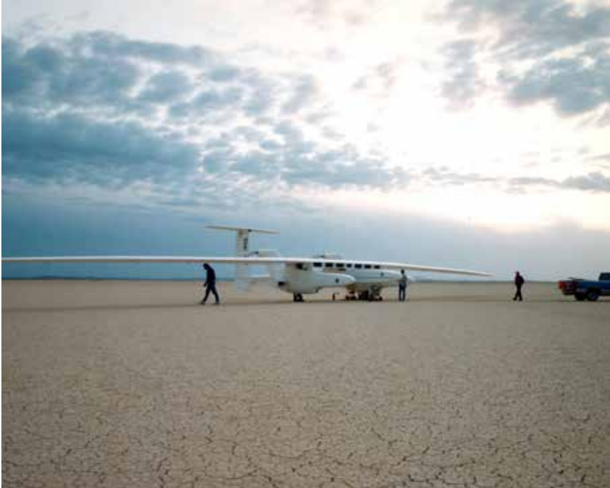
The Theseus was a high-altitude, long-endurance vehicle capable of carrying a 700-pound payload to 60,000 feet. NASA
