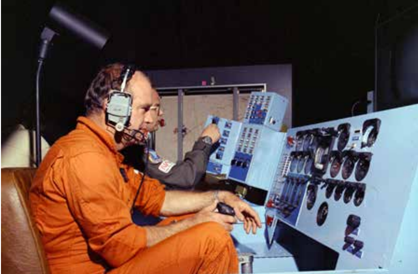
Bill Dana, foreground, controls the HiMAT from the ground cockpit while a flight-test engineer monitors the aircraft's systems. NASA
