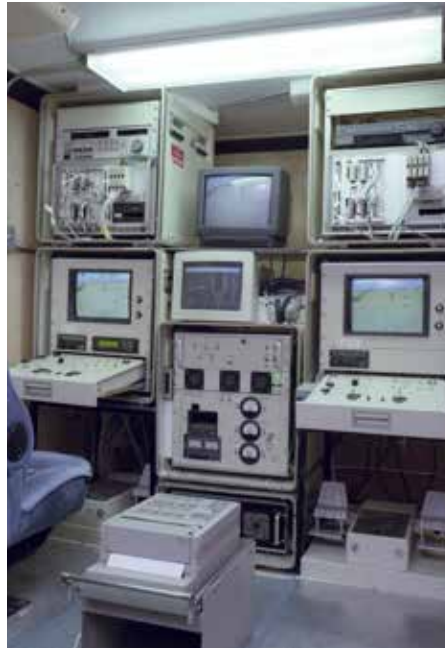
The Perseus ground control station contained simple joystick and switch controls, ground-track/location monitor, head-up display, and flight instruments displayed on CRT screens. NASA
