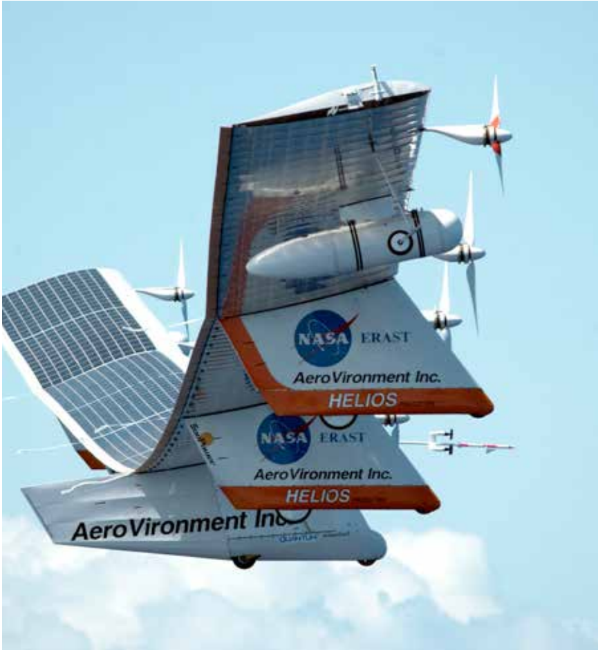
The Helios Prototype in flight, demonstrating normal dihedral conditions. NASA
