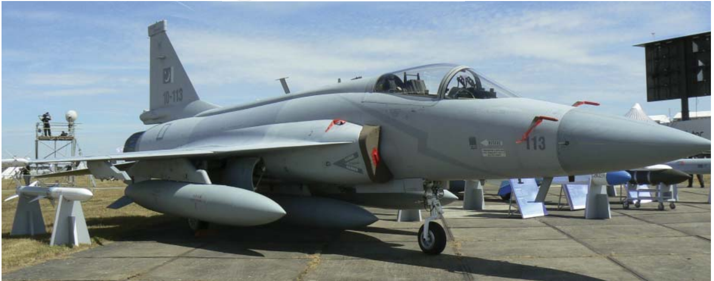
CAC/PAC JF-17 Thunder lightweight combat aircraft jointly developed by China and Pakistan. Chris Male photo.
