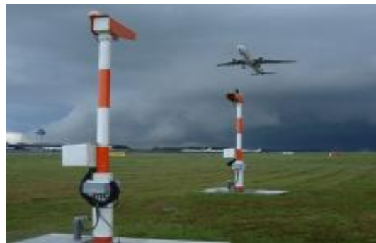
Vaisala MITRAS 18 Transmissometer sensor mast and array (Vaisala company Oyj, PO Box 26 00421 Helsinki, Finland)
