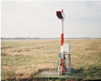
Vaisala MITRAS 18 Transmissometer sensor mast and array (Vaisala company Oyj, PO Box 26 00421 Helsinki, Finland)
