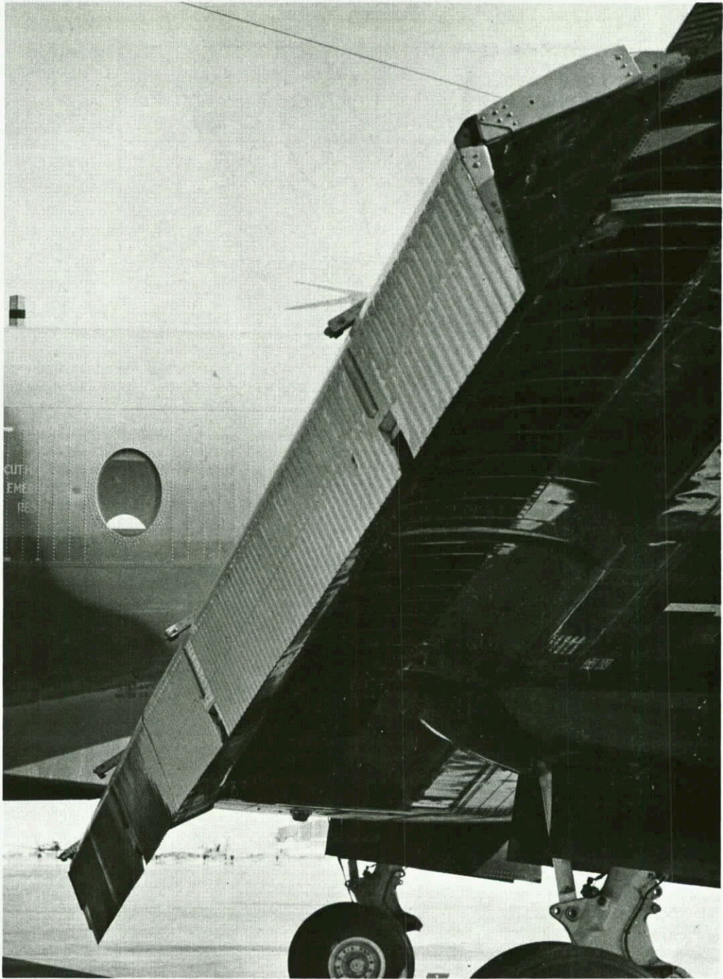
Fig.3 Andover C. Mk.1. Flap/tab in S.T.O.L. landing position
