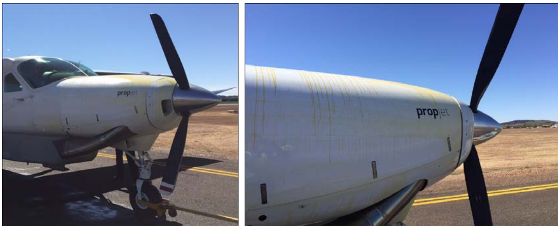
Figure 1: Photographs of VH-LNH after the aircraft had landed, with oil visible on the engine cowl and forward fuselage
