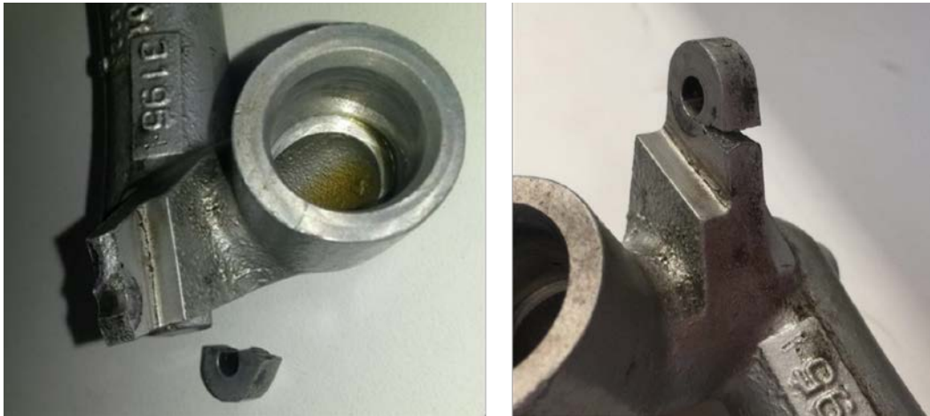
Figure 4: Fractured lug (the figure on the right shows that a segment of the lug was missing)
