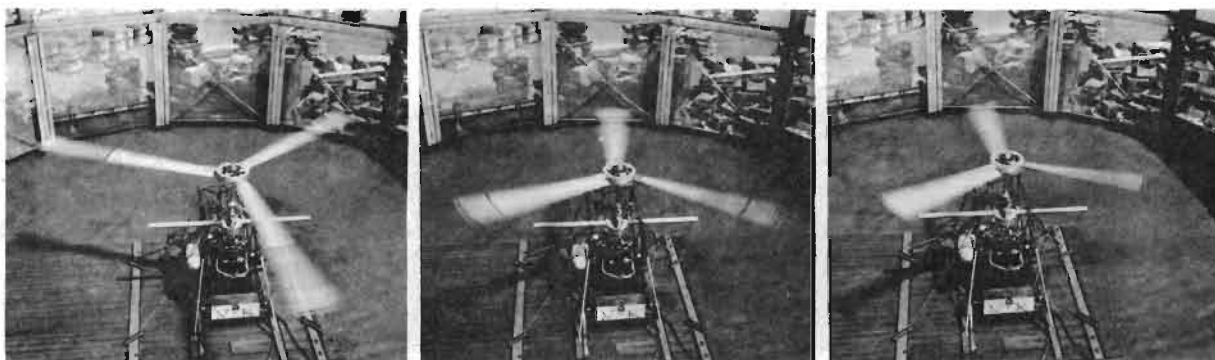
FIGURE 15. VARIABLE-DIAMETER ROTOR TEST SHOWING CONTRACTION TO 60% DIAMETER
